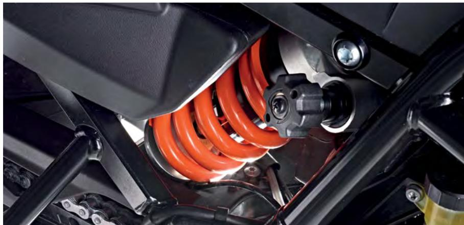
After the successful introduction of the ESA in Boxer and K-models many years ago BMW now decided to create a Mini-ESA version for the smaller models F 700 / F 800 GS. Here the rider has the option to change the damping in the three steps soft, medium or sport at the push of a button at the handlebars!
