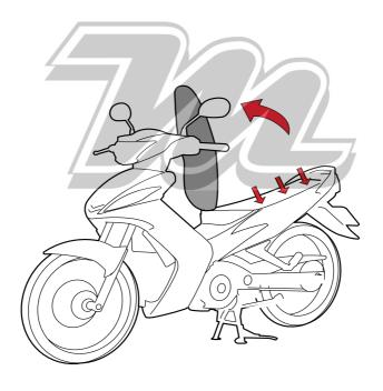
Remove the rear tail lamp cowl by loosening the two screws.
