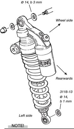
The shock absorber shall be mounted with the cylinder head upwards and the reservoir backwards. Use the supplied washers and sleeves to fit the shock absorber on your bike.
