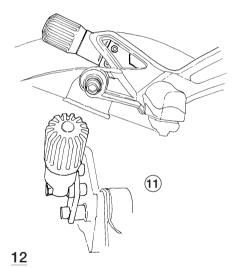
Mount the adjuster and let the hose go in soft turns to the spring preloder. Fix the hose with tie-raps.
