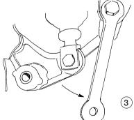
Loosen first the lower shock absorber attachment then the upper shock absorber attachment.
