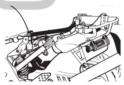
On this model is an adjustable end eye/ bracket mounted. The end eye/bracket must not be threaded out more than that the groove is visible beneath the locknut. See fig. Make sure that the locknut is tightened after adjustment.
