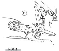
Make sure that all bolts are tightened to the correct torque and that nothing fouls or restricts movement of the shock absorber when the suspension is being fully compressed or extended.
