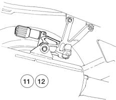
Let the hose go in soft turns to the spring preloder. Fix the hose with tie-raps.
