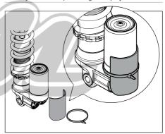
Tighten the upper and the lower attachments. Make sure that all removed parts are installed in the same way as they were before the installation.
