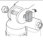
Install the Öhlins shock absorber in the same way as the original unit. Use the original attachment screws.
