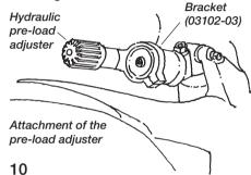
Fit the pre-load adjuster so that the hose is smoothly curved.
