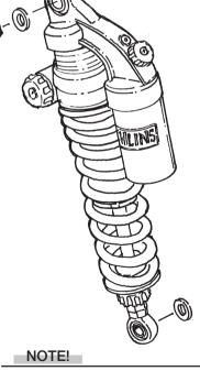
The shock absorber shall be mounted with the cylinder head upwards and the reservoir backwards. Use the supplied washers and sleeves to fit the shock absorber on your bike.
