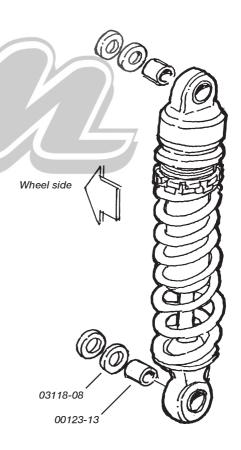
Normaly the shock absorber is mounted with the cylinder head upwards. Check that there is enough clearence to other details both in loaded and unloaded position.
