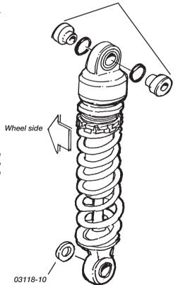
Normaly the shock absorber is mounted with the cylinder head upwards. Check that there is enough clearence to other details both in loaded and unloaded position.
