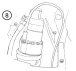
Attach the shock absorber to the upper bracket.
