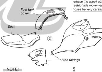
The screws holding the fairings are of different lengths. Make sure to return them to the correct position.
