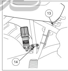
Reinstall the chain guide, plastic cover, electrical connector and the seat. Make sure that all removed parts are reinstalled in the same way as they were before the installation.
