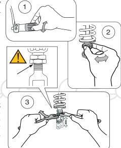
upper nut with one hand and at the same time loosen the lock nut (lower nut). Turn the end eye/ bracket to the desired length. Lock the lock nut. Tightening torque: 40 Nm
