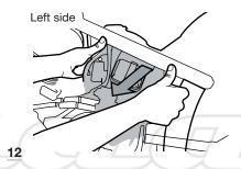
Remove the original shock absorber.
