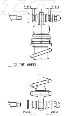
On the left side the gas valve shall be pointing forward.
